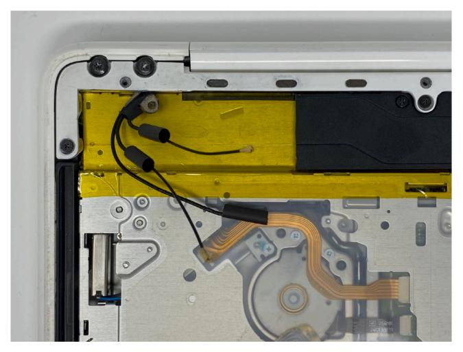
d. Carefully slide the heat shrink over the connectors and shrink them either using a hot air gun or hair dryer.
