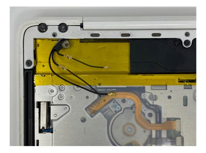
c. Cut 1cm lengths of **BLACK** heat shrink and slide these onto the antenna cables.
