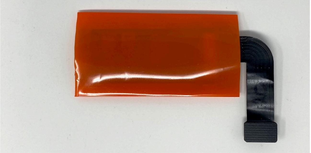
b. Carefully trim the heat shrink to expose the antenna connectors on the top side of the WiFi card.
