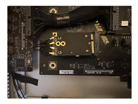
**6. Install the WiFi Card and Adaptor**Now turn the card over carefully so as not to disconnect the antenna cables install the WiFi Card and Adaptor in the Mini PCIe slot and secure with a single screw.
